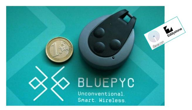
The device brings together the ability of the BLE to automatically transmit data and user's voluntary activities: the three buttons are designed to transmit different types of information such as location based services or voluntary events (automation, access control, help, safety at work...).
